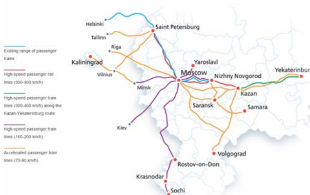
Plan for the introduction of rapid, high-speed and super high-speed passenger trains prior to Russia hosting the FIFA World Cup in 2018:
